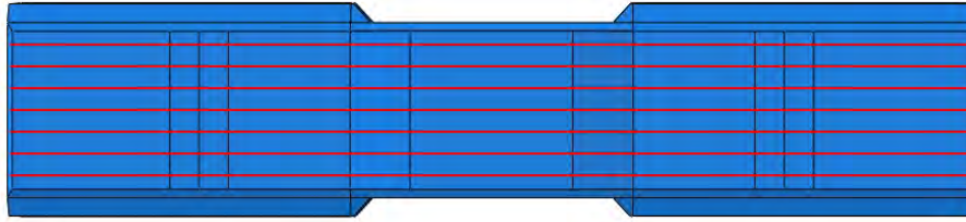
Fig. 15. PC tendon design of the FE model
