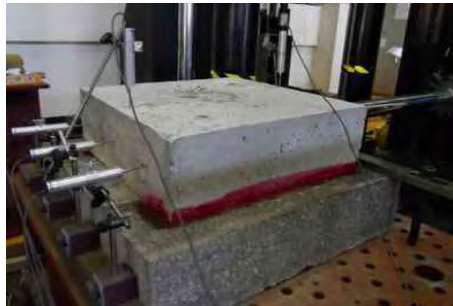
Fig. 1. Experimental test of frictional force between asphalt-concrete structures
