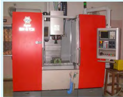
Fig. 1 CNC Vertical Machine Centre
