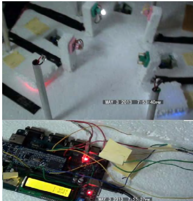
Lane 1 Slot 2 and Lane 2 Slot 2 are occupied and the next incoming car is allotted lane 1 slot 1.
