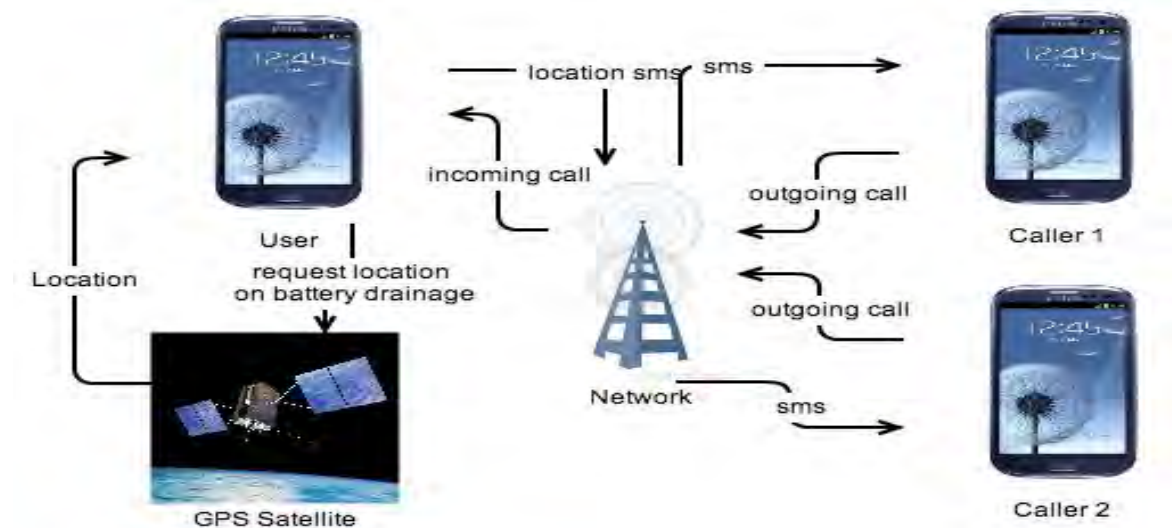
Figure 1: System Architecture of Location SMS to Incoming Number on Battery Drainage
