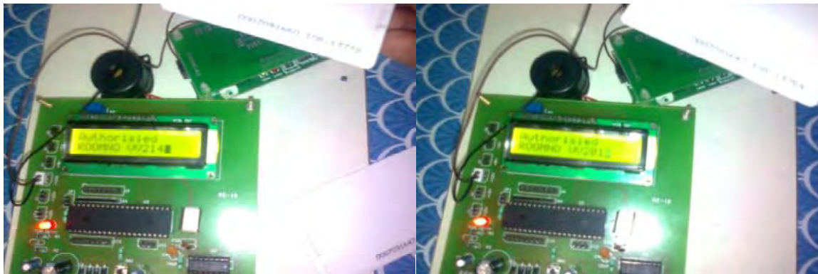
Figure 4 Protype model with the student register number on the LCD
