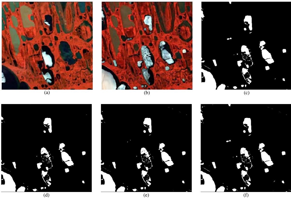
Fig.4 Change detection results obtained from different methods (a) Landsat 5 Image acquired on July 22, 1985 (b) Landsat 5 Image acquired on July 13, 2005 (c) Ground truth of change detection (d) PCA-based approach (e) NSCT method (f) Proposed Method
