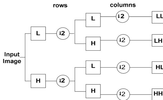
Fig.2 One Step Decomposition using DWT
