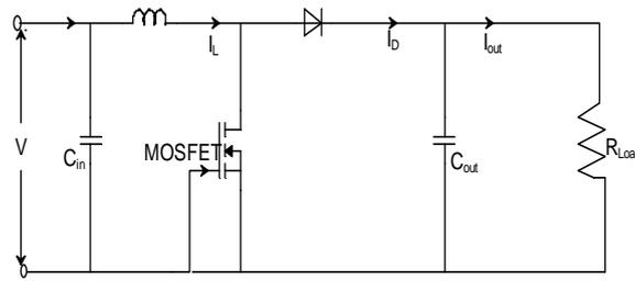
Fig. 3. Boost DC/DC converter
