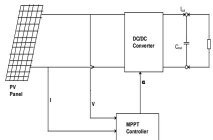
Fig. 1. Block diagram of the PV system
