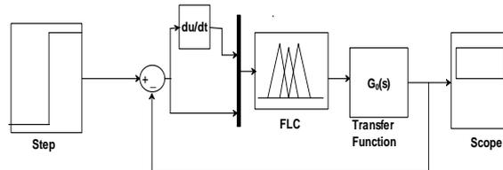
Fig. 8. Simulink model of MPPT using fuzzy logic controller.
