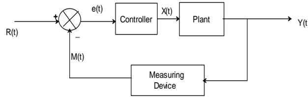
Fig. 4. General block diagram of a closed loop system
