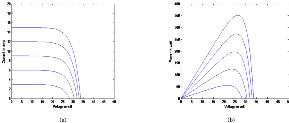
Fig. 9. (a) I-V characteristics (b) P-V characteristics
