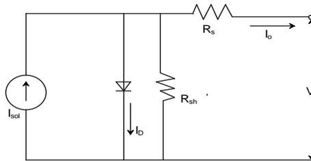
Fig. 2. Circuit configuration of the PV panel
