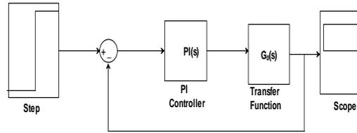
Fig. 7. Simulink model of MPPT using PI controller
