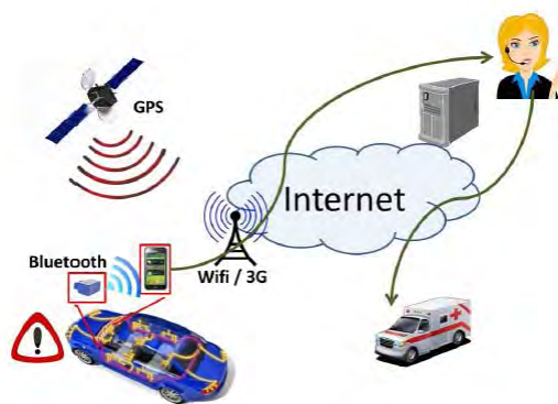
Fig. 3. Improved application of embedded systems in vehicles based on smartphones [14]
