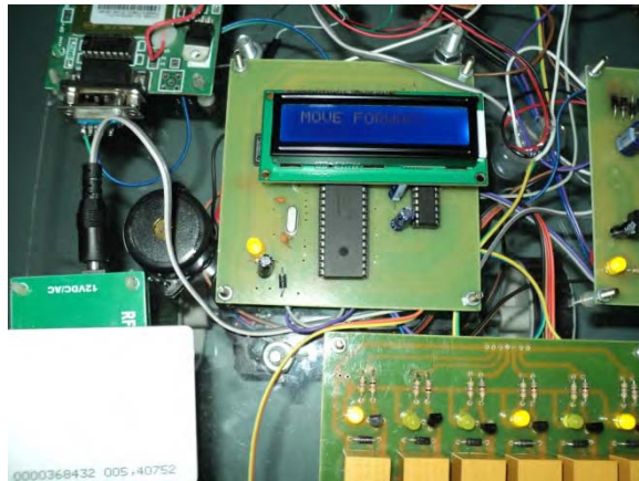
Fig. 7: Vehicle moves forward with help of RFID tag
