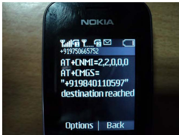
Fig. 17: Destination reached message to control station
