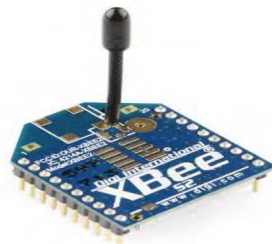
Fig. 6 Xbee module for wireless communication
