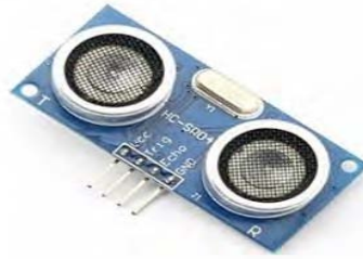
Fig.4 Robot sensors edifice (ultrasonic sensor)
