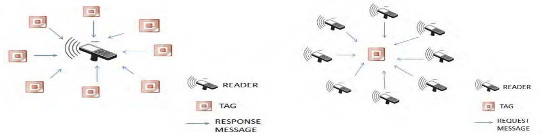
Fig1.RFID Collision: (a) Tag Collision (b)Reader Collision
