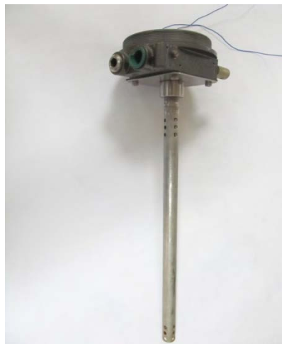
Fig. 2. Coaxial Capacitive Sensor used in the System
