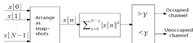
Fig 1. Energy detector block diagram
