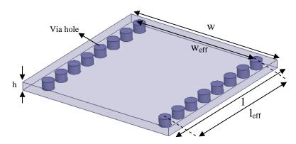
Fig. 2. Basic structure of SIW
