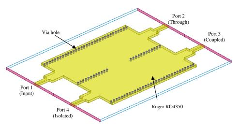
Fig. 1. Configuration of X-Band SIW directional coupler
