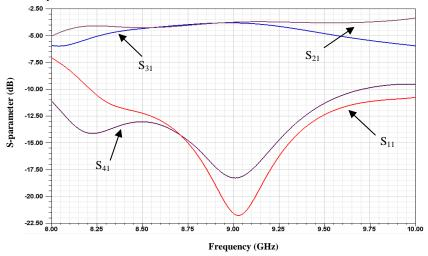
Fig. 5. S-parameter of X-band SIW directional coupler
