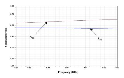
Fig. 6. The magnitude of  $S_{21}$  and  $S_{31}$
