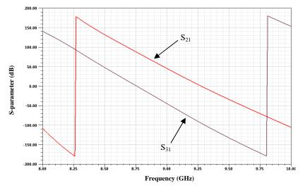
Fig. 7. Simulated phase of coupled wave in Port 2 and Port 3
