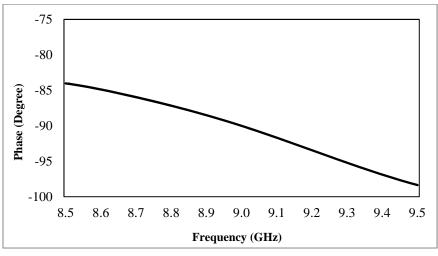
Fig. 8. The phase difference between two coupled ports
