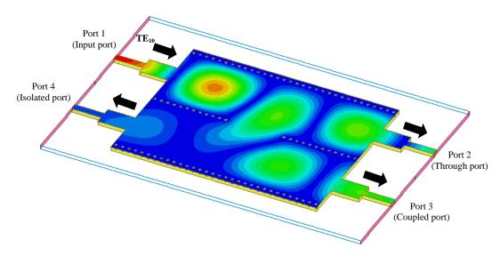
Fig. 9. Magnetic E-field of SIW directional coupler
