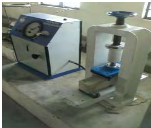
Fig. 4. Test set up for flexural strength testing machine
