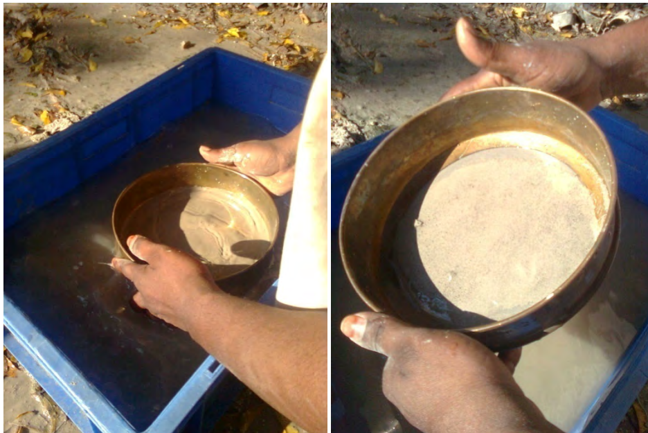
Fig. 1. Wet sieving for fineness of fly ash
