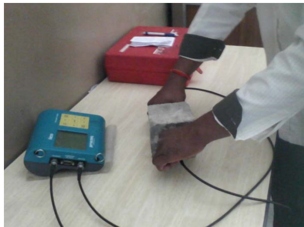
Fig. 11. Ultrasonic pulse velocity test set up
