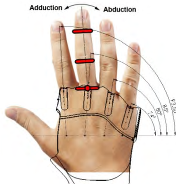
Fig. 4. Schematic showing placement and angular degree of freedom of the orthosis joints overlaid on a human hand
