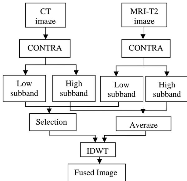
Figure 6. Block diagram of Contourlet Transform
