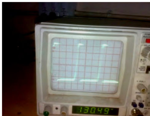
Figure5.4: Voltage waveform across the switch ( V_{DS} ).
