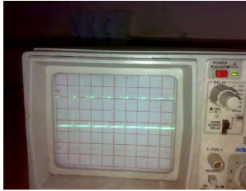
Figure5.3: Waveform across the secondary winding of a transformer.
