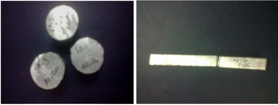
Fig. 2- Brinell hardness and Impact strength Tested Specimen.
