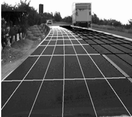
Fig 4. Left corner and side lane detected on highway
