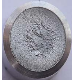
Fig.2. Cross sectional view of a fatigue failed CCRB specimen
