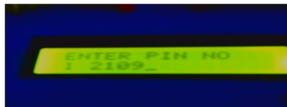
Fig. 9. Employ code displaying on LCD
