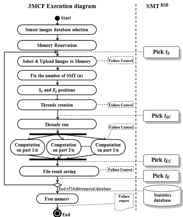
Fig. 3. 3MCF execution diagram and SMT<sup>RSB</sup> picked time positions. *t<sub>S</sub>*, pick time for start image computation, *t<sub>SC</sub>*, pick time for start core computation, *t<sub>EC</sub>*, pick time for end core computation, *t<sub>E</sub>*, pick time for end image computation
