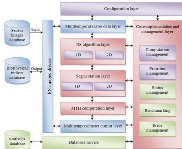
Fig. 2. Core framework architecture diagram.
