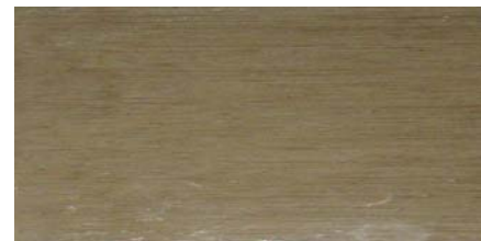
Fig. 9. Prepared cotton-polyester composite plate
