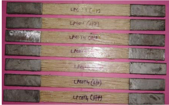
Fig. 10. Prepared cotton-polyester composite specimen for testing
