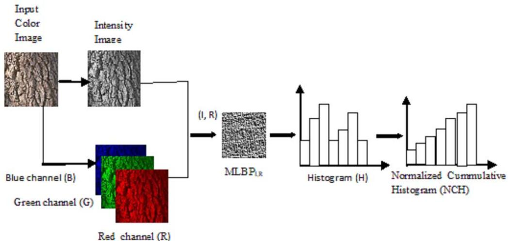
Figure 4. Schematic diagram of the proposed color texture feature extraction using MLBP method.
