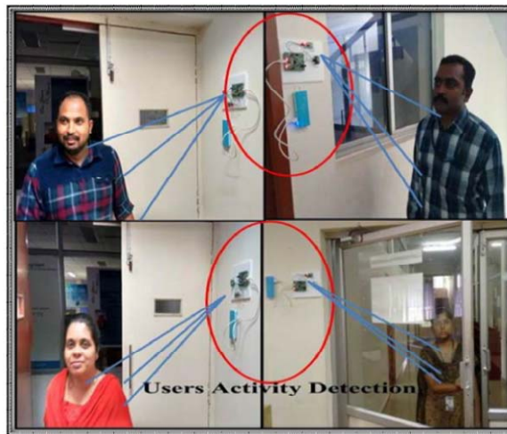
Figure 8. Real time users' activity signals detected using PIR sensor
