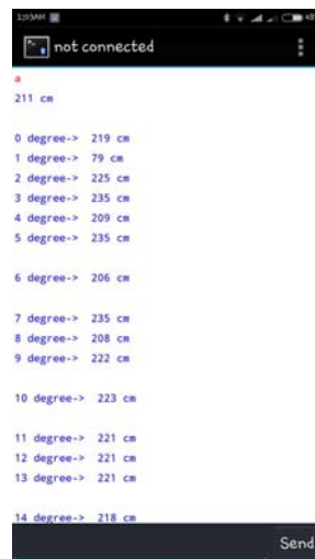
Figure 9. Data collected by sensor received on a bluetooth enabled device (android) via bluetooth module HC-05
