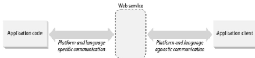
Figure 2. Web services providing an abstraction layer between the application client and its code
