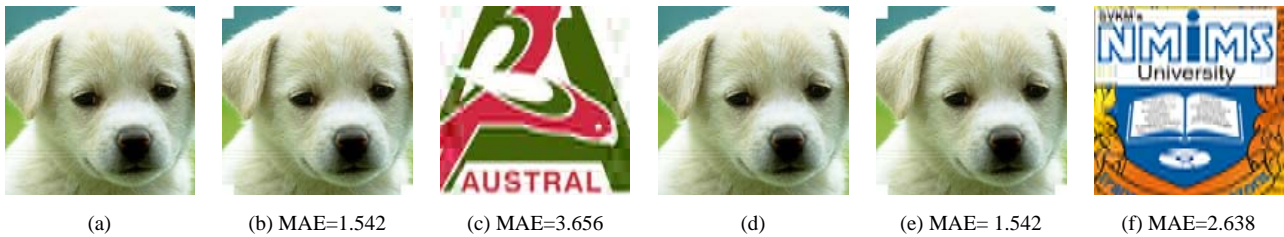
Figure 9. Result images for cropping 16x16 squares at four corners of watermarked image (a) 'Puppy' watermarked with 'austral' (b)watermarked 'Puppy' after cropping 16x16 square at four corners (c)extracted watermark 'austral' from cropped 'puppy' (d) 'Puppy' watermarked with 'nmims' (e) watermarked 'Puppy' after cropping 16x16 square at four corners (f) extracted watermark 'nmims'
