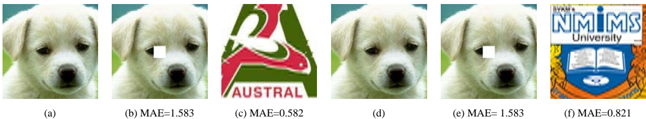
Figure 11. Result images for cropping 32x32 squares at centre of watermarked image (a) 'Puppy' watermarked with 'austral' (b)watermarked 'Puppy' after cropping 32x32 square at centre (c)extracted watermark 'austral' from cropped 'puppy' (d) 'Puppy' watermarked with 'nmims' (e) watermarked 'Puppy' after cropping 32x32 square at centre (f) extracted watermark 'nmims'
