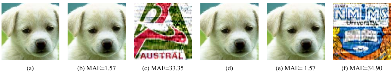
Figure 7. Result images for compression of watermarked image using column Walsh transform (a) 'Puppy' watermarked with 'austral' (b)watermarked 'Puppy' after compression (c)extracted watermark 'austral' from compressed 'puppy' (d) 'Puppy' watermarked with 'nmims' (e) watermarked 'Puppy' after compression (f) extracted watermark 'nmims' from compressed 'puppy'
