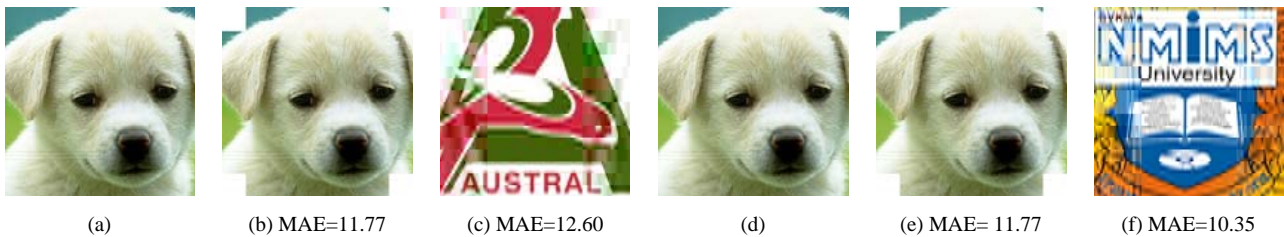
Figure 10. Result images for cropping 32x32 squares at four corners of watermarked image (a) 'Puppy' watermarked with 'austral' (b)watermarked 'Puppy' after cropping 32x32 square at four corners (c)extracted watermark 'austral' from cropped 'puppy' (d) 'Puppy' watermarked with 'nmims' (e) watermarked 'Puppy' after cropping 32x32 square at four corners (f) extracted watermark 'nmims'
