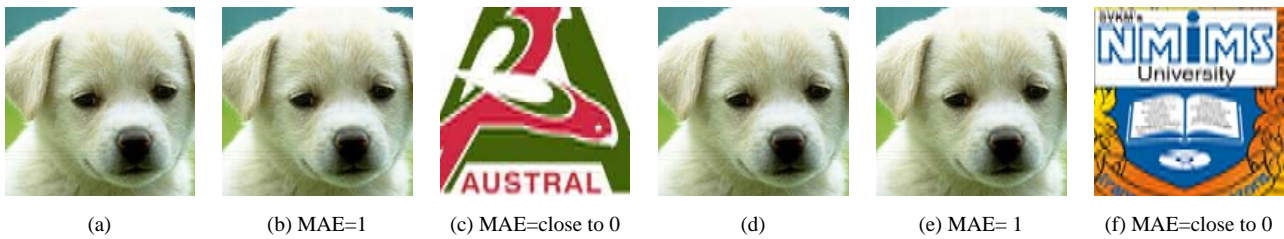
Figure 12. Result images for binary distributed run length noise added to watermarked image (a) 'Puppy' watermarked with 'austral' (b)watermarked 'Puppy' after adding noise (c)extracted watermark 'austral' from noise added 'puppy' (d) 'Puppy' watermarked with 'nmims' (e) watermarked 'Puppy' after adding noise (f) extracted watermark 'nmims' from noise added 'puppy'
