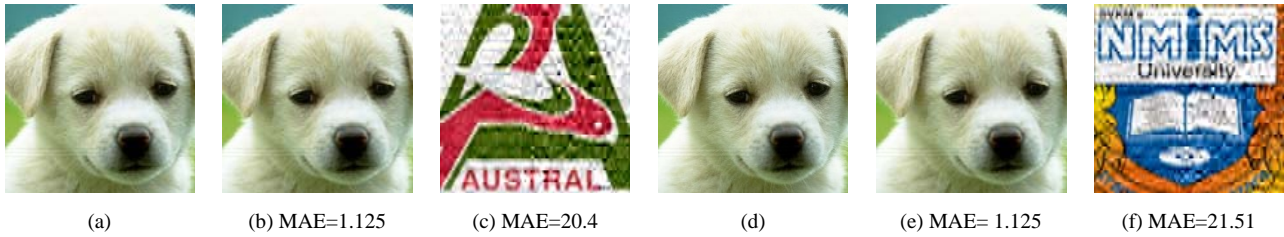
Figure 14. Result images for Type 1 image resizing attack on watermarked image (a) 'Puppy' watermarked with 'austral' (b)watermarked 'Puppy' after resizing (c)extracted watermark 'austral' from resized 'puppy' (d) 'Puppy' watermarked with 'nmims' (e) watermarked 'Puppy' after resizing (f) extracted watermark 'nmims' from resized 'puppy'
