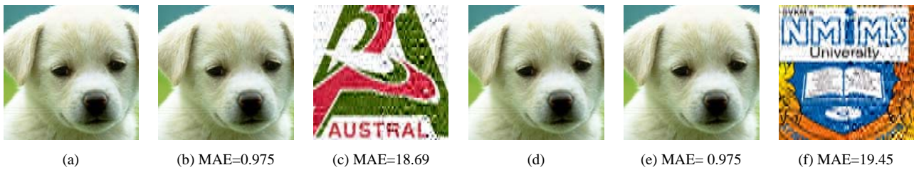
Figure 5. Result images for compression of watermarked image using column DCT transform (a) 'Puppy' watermarked with 'austral' (b)watermarked 'Puppy' after compression (c)extracted watermark 'austral' from compressed 'puppy' (d) 'Puppy' watermarked with 'nmims' (e) watermarked 'Puppy' after compression (f) extracted watermark 'nmims' from compressed 'puppy'
