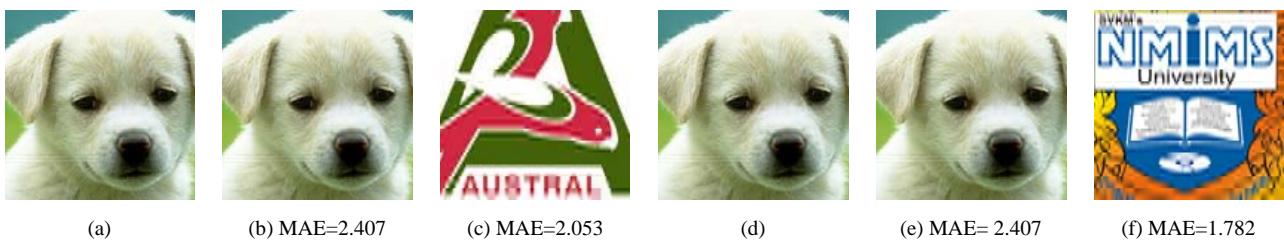
Figure 4. Result images for compression attack with compression ratio 1.95 (a) ‘Puppy’ watermarked with ‘austral’ (b)watermarked ‘Puppy’ after compression (c)extracted watermark ‘austral’ (d) ‘Puppy’ watermarked with ‘nmims’ (e) watermarked ‘Puppy’ after compression (f) extracted watermark ‘nmims’
