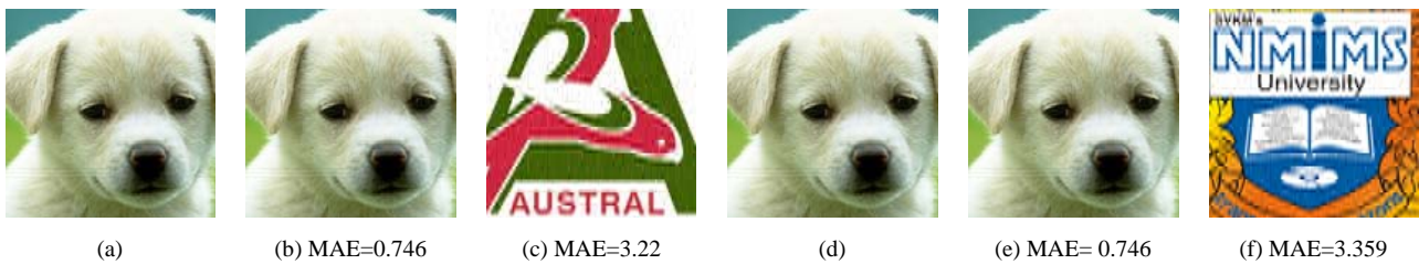
Figure 13. Result images for Gaussian distributed run length noise added to watermarked image (a) 'Puppy' watermarked with 'austral' (b)watermarked 'Puppy' after adding noise (c)extracted watermark 'austral' from noise added 'puppy' (d) 'Puppy' watermarked with 'nmims' (e) watermarked 'Puppy' after adding noise (f) extracted watermark 'nmims' from noise added 'puppy'
