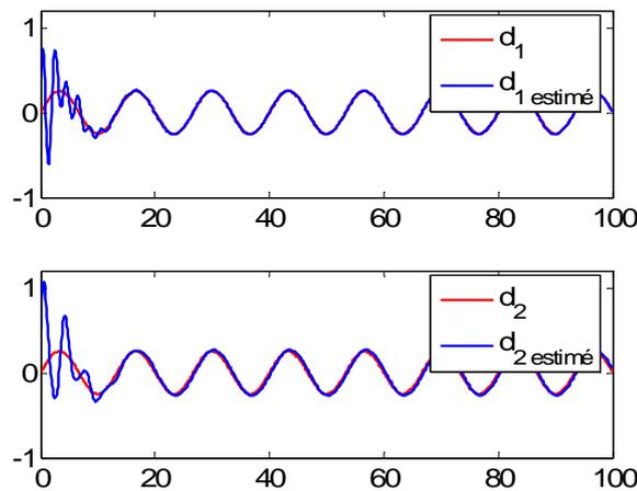
Fig.2 Actuator fault and its estimation
