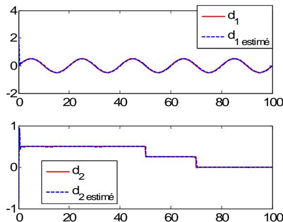
Fig.10 Actuator faults and their estimations
