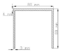
Material to be used for cast piston Al-Si= $\sigma_s$ =47.000 psi. **Molten-Metal Volume** Volume of cast product Volume=( $\pi/4$ )(80<sup>2</sup>)(80)- ( $\pi/4$ )(74<sup>2</sup>)(76)= 23956  $\pi$  mm<sup>3</sup> Total volume of molten metal V<sub>m</sub>=23977 $\pi$  mm<sup>3</sup> **Sprue volume**
