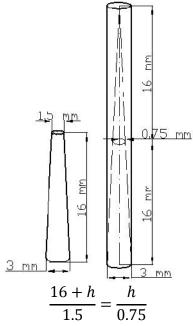
1.5h=16(0.75)+0.75h 0.75h=16(0.75)=12 h=16  $V_1=1/3\pi r^2(32)-1/3\pi r^2(16)=24\pi - 3\pi = 21\pi$ . Let the ram's stroke be 3d Where= $r^2/2$ ,  $r^2 =>$  internal diameter of the piston.
