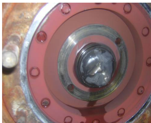
Figure n°4: Shear of shaft
