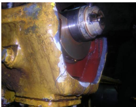
Figure n°3: Failure of bearing
