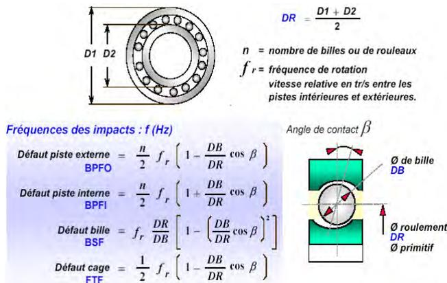
Figure 4. Frequency characteristics of the defects of elements of a bearing
