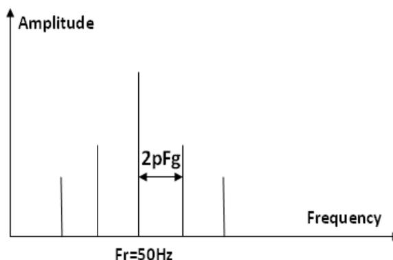
Figure 17.spectre of the motor with a rotor defect
