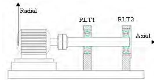
Figur7. Layout of the test bench realized
