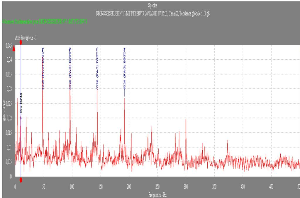
Figure 21. Envelope spectre at point (P2) of the motor
