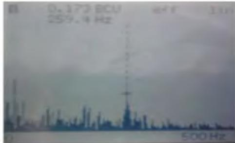
Figure 8. Envelope spectre of the Bearing breast
