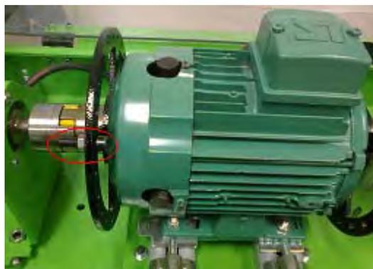
Figure 12.picture of the motor with Unbalance fault
