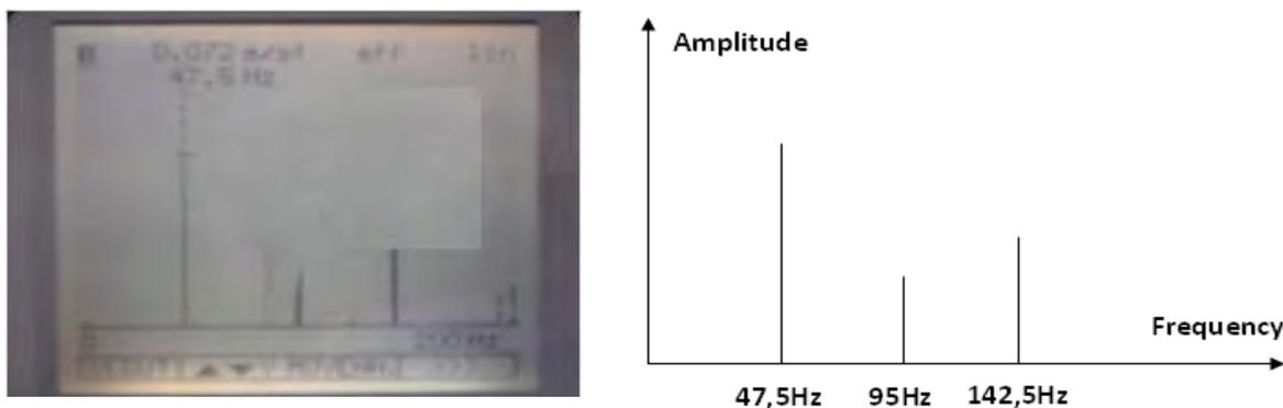
Figure 13.Spectre for the Unbalance fault
