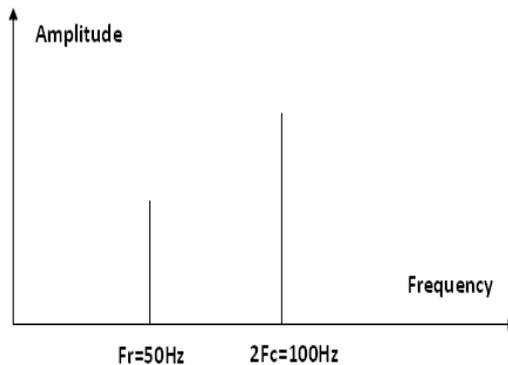
Figure 15.spectre of the motor with a stator defect
