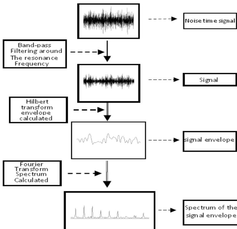
Figure 3: Principle of the envelope analysis [12]
