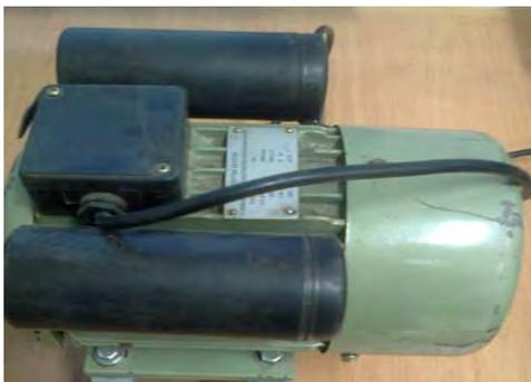
Figure 14.picture of the motor with a stator defect
