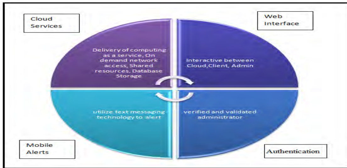
Figure1. Modules of Integral System.
