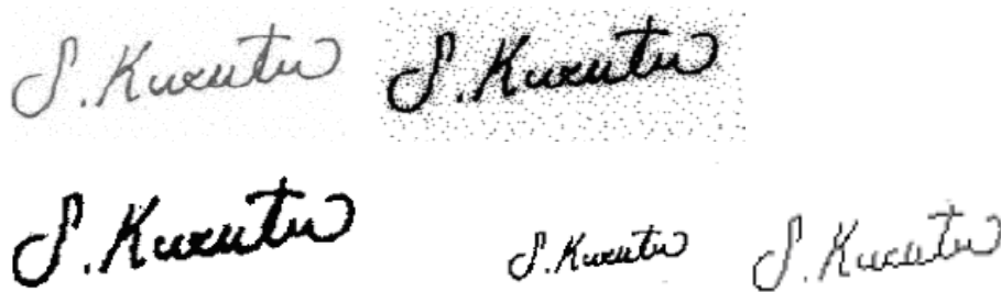
Fig 3. Preprocessing steps: (a) scanning, (b) background elimination, (c) noise reduction, (d) width normalization, (e) thinning applied signatures.
