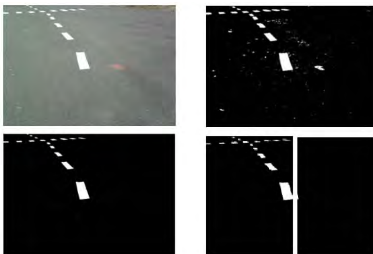
Figure 8. Frame processing for lane following.
