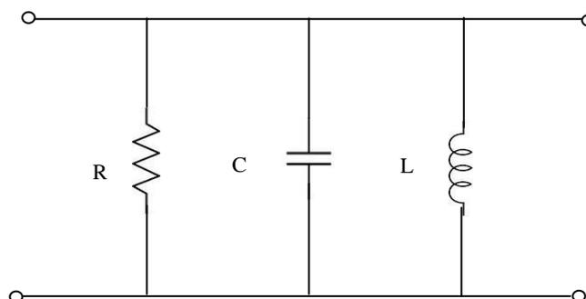
Figure2: Equivalent circuit of Annular Ring Microstrip Antenna
