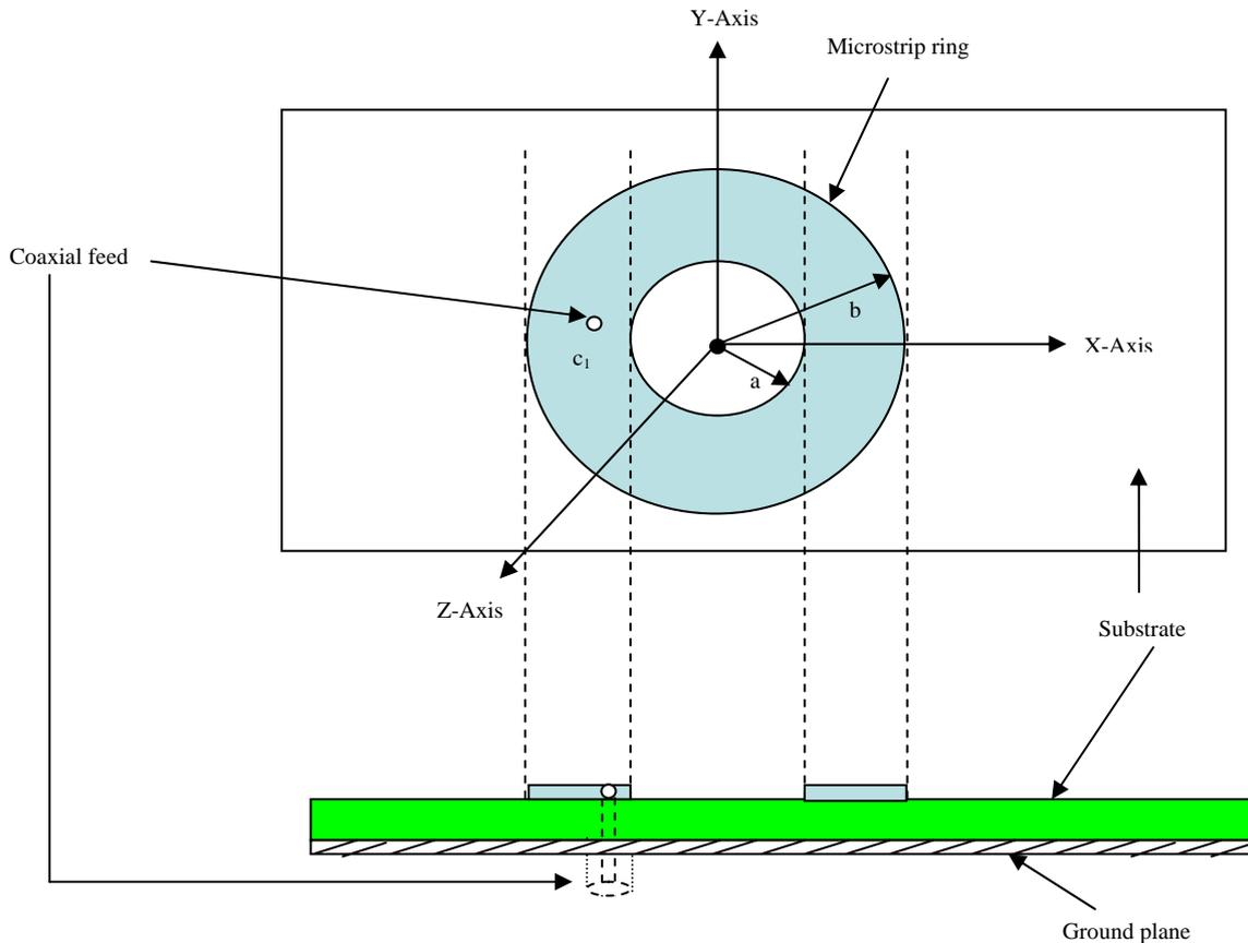
Figure1: Annular Ring Microstrip Antenna
