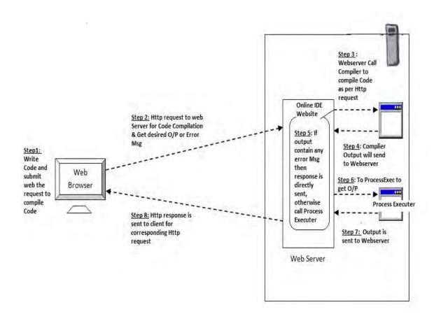
Figure 1 Architecture of Web-Based 'C' IDE
