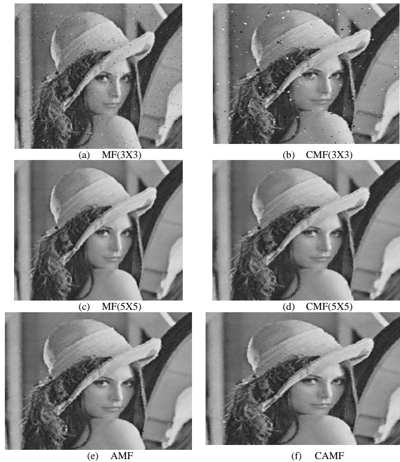
Figure8. Shows outputs of different filters for 250X250 Lena image at noise density 30%
