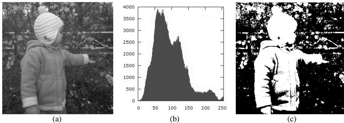
Figure 2. (a)Kid image, (b) histogram, (c) thresholded image.
