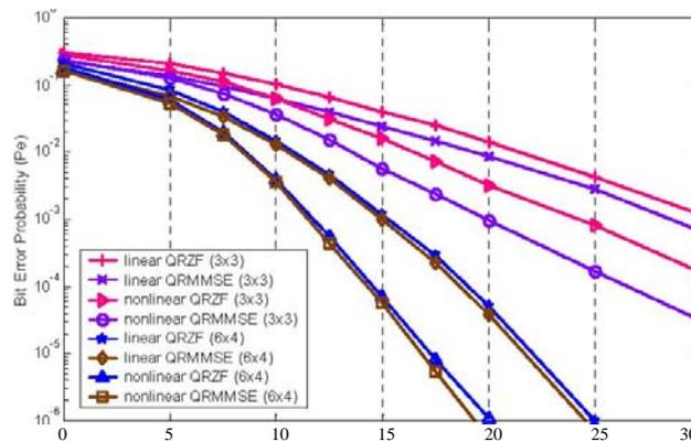
Fig. 3: System performance for the  $(6 \times 4)$  &  $(3 \times 3)$  system configuration for both linear and nonlinear QR detection using either ZF or MMSE criteria.
