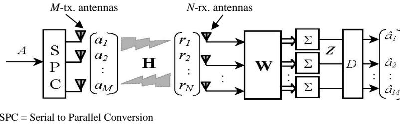
Fig.1: Space-time system model with symbol detection.
