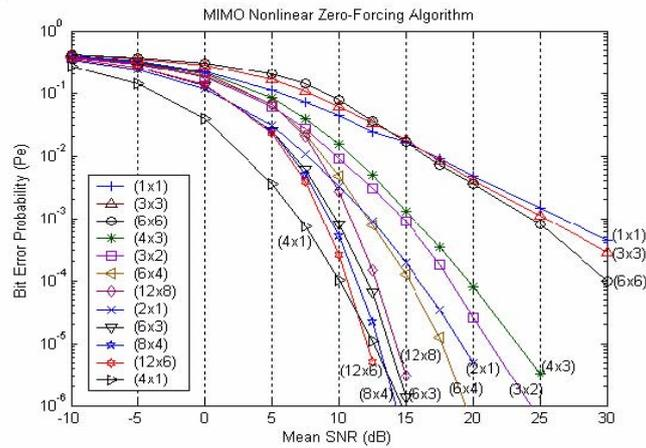
Fig. 7: Performance of layered space-time receiver using nonlinear ZF algorithm.
