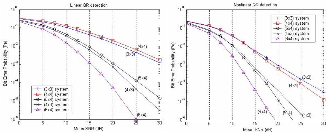
Fig. 2: Bit Error Performance using linear QR & nonlinear QR method.
