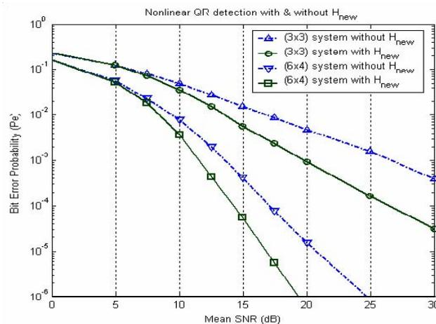
Fig. 4: System performance using nonlinear QR detection a) with  $\mathbf{H}_{new}$  & b) without  $\mathbf{H}_{new}$
