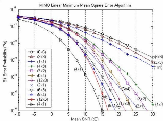
Fig. 6: Performance of layered space-time receiver using linear MMSE algorithm.
