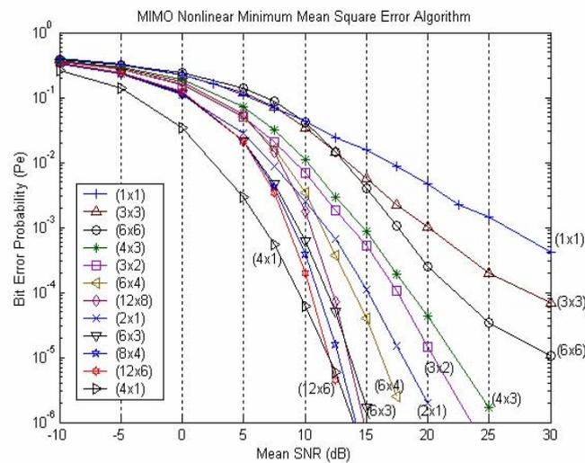
Fig. 8: Performance of layered space-time receiver using nonlinear MMSE algorithm.
