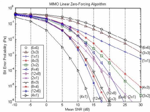
Fig. 5: Performance of layered space-time receiver using linear ZF algorithm.
