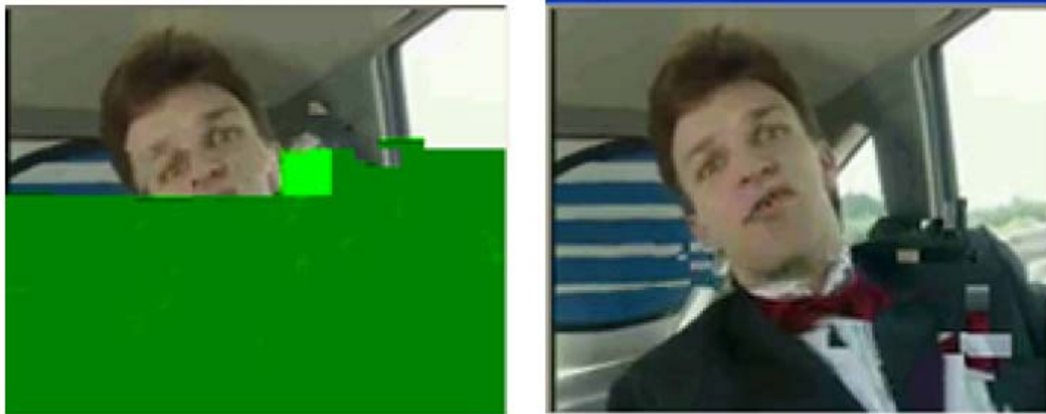
Fig 10: Comparison of subjective reconstructed video quality for Carphone video sequence at SNR=22.0dB in 64kbps; (a) UEP-PPS-QAM the proposed scheme; (b) Non-PPS-UEP-1 scheme from [8];
