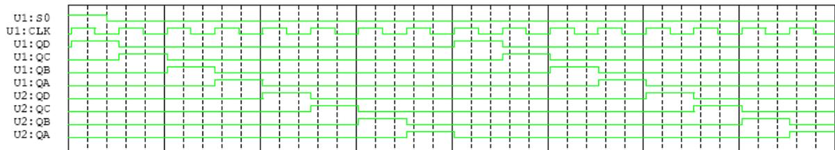
Figure 4. Waveforms obtained at the output of the ring counter
