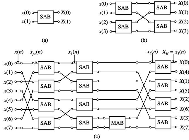
Figure 6. Analog block structure to obtain the DHT for (a)  $N = 2$ , (b)  $N = 4$  and (c)  $N = 8$
