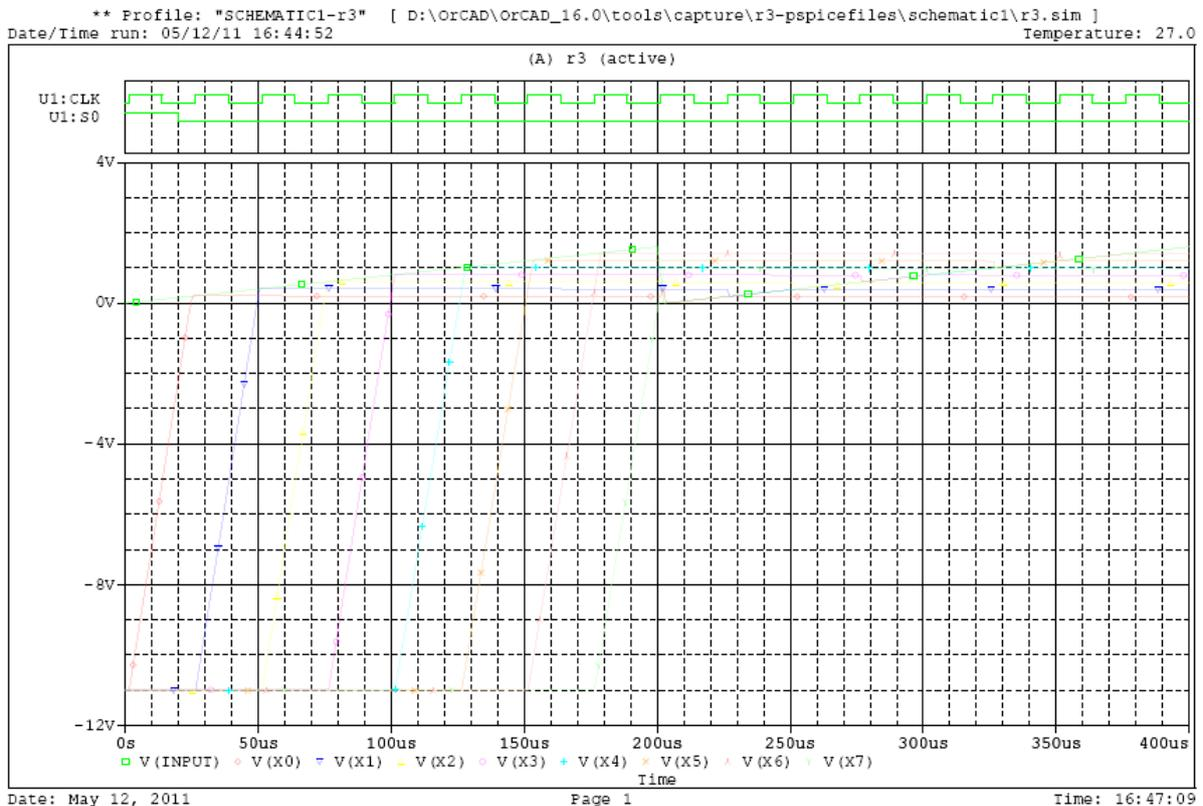
Figure 5. Waveforms obtained at the output of the sample and hold array
