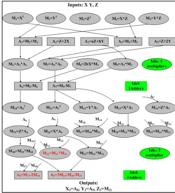
Figure 3: The 5-PM design for Binary Edwards ECC for point doubling operation over GF (P) using Projection (X/Z, Y/Z).
