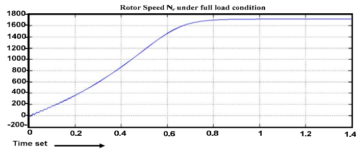
Fig. 12. Rotor Speed N_r under full load condition n_s=1714 , t_s=0.89
