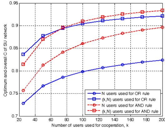
Figure 13. Optimum and overall normalized capacity versus variable fraction (k) of different total number of users under CPUP scenario.
