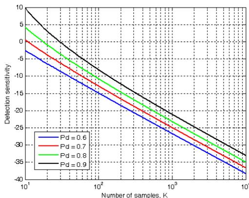
Figure 2. Detection sensitivity versus number of samples under CPUP scenario
