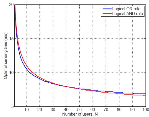
Figure 9. Optimal sensing time versus number of collaborated users under CPUP scenario.
