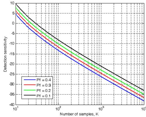
Figure 3. Detection sensitivity versus number of samples under CSUSU scenario
