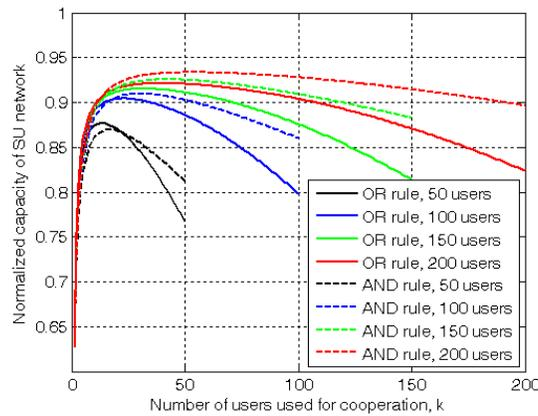
Figure 12. Normalized capacity versus variable fraction ( $k$ ) of different total number of users ( $N = 50, 100, 150,$  or 200) under CPUP scenario.
