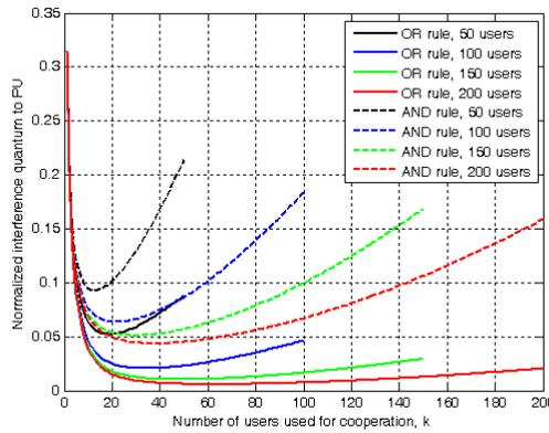
Figure 14. Normalized capacity versus variable fraction (k) of different total number of users ( $N = 50, 100, 150,$  or  $200$ ) under CSUSU scenario.
