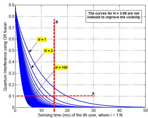
Figure 10. Quantum Interference versus sensing time with different number of users using OR-rule fusion scheme under CSUSU scenario.
