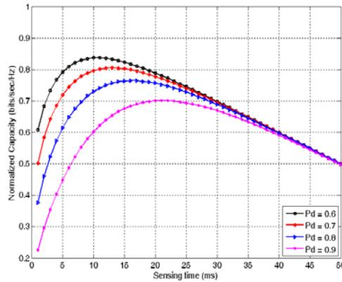
Figure 6. Normalized capacity versus sensing time for local sensing under CPUP scenario.
