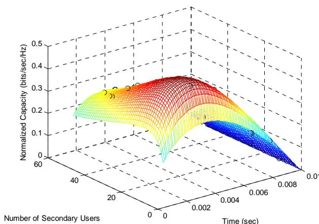
Figure 17. Normalized capacity as a function of sensing time and number of secondary users.
