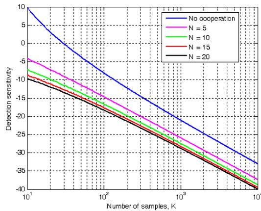
Figure 4. Detection sensitivity versus number of samples with different number of samples ( $P_d = 0.9$  and  $P_f = 0.1$ )
