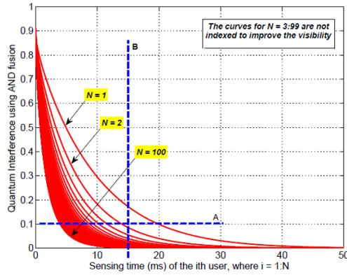
Figure 11. Quantum Interference versus sensing time with different number of users using AND-rule fusion scheme under CSUSU scenario.
