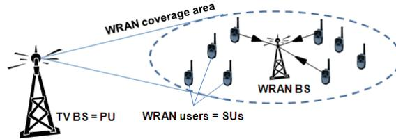
Figure 1. IEEE 802.22 WRAN system deployment.
