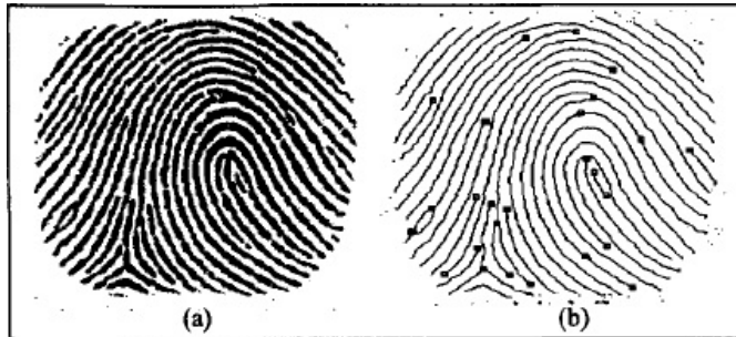
Figure 2: (a) Original fingerprint. (b) Detected minutiae.
