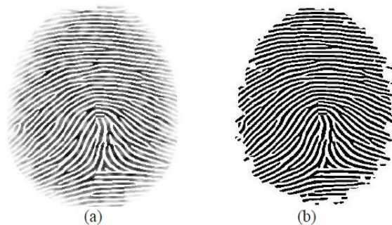
Figure 10: (a) Original Fingerprint, (b) Binarized Fingerprint.
