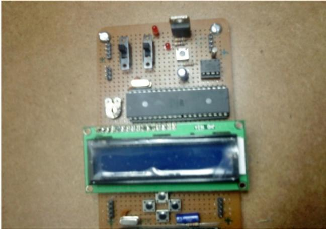
Fig 3 Interfaces to Microcontroller M1
