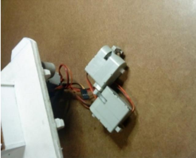
Fig 7 Leg design with two servos
