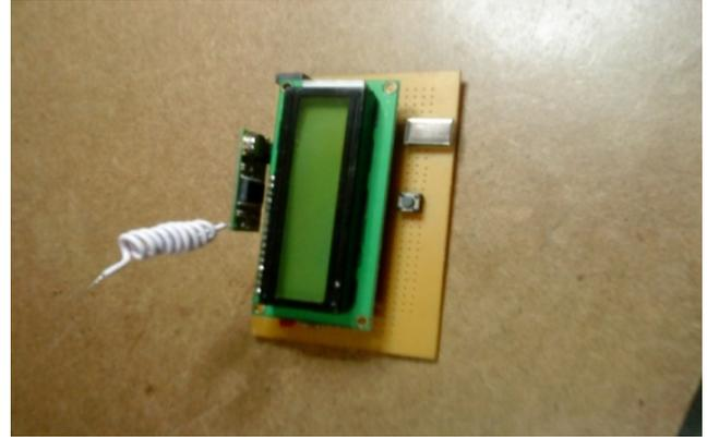
Fig 5 Microcontroller M3 with RF receiver
