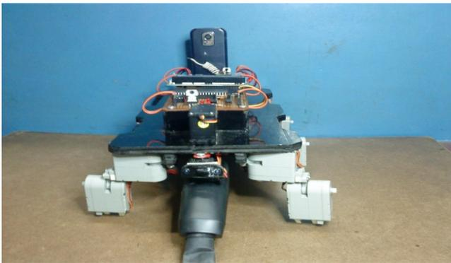
Fig .1 Autonomous Hexapod Robot
