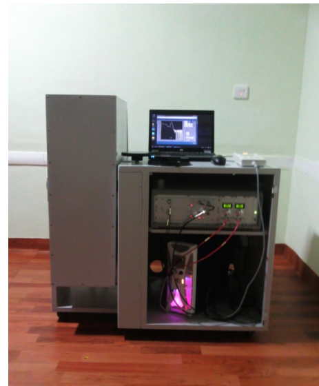
Fig.1 The photograph of Compact Dual Polarization Lidar The CDPL is an independent custom-built system that housed in a movable construction. Fig. 1 shows the photograph of the
