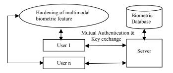
Figure 1. Architecture for multimodal biometric authentication
